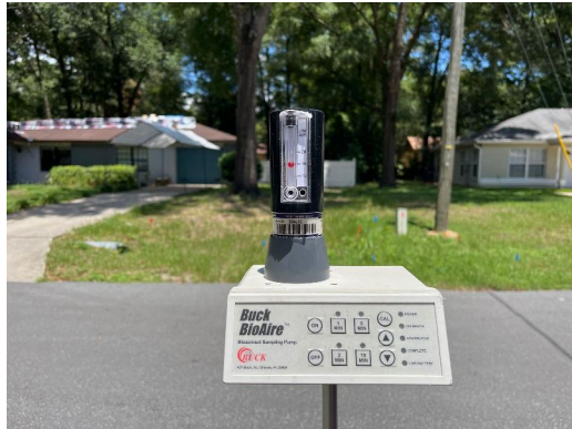
Calibration prior to testing
